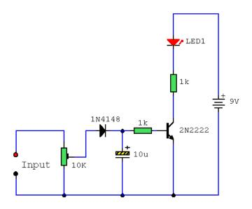
Operation is the same as the op-amp circuit. The input is now directly to a 10k preset resistor, the monitored audio signal being half-wave rectified and used to directly bias the transistor. As before any transistor with a forward dc current gain greater than 100 may be used.
